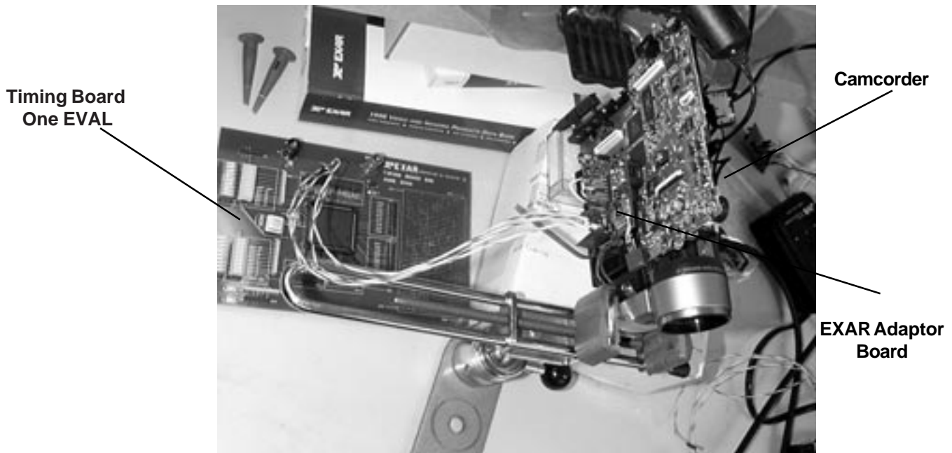
Figure 3. Timing Board One EVAL (Serial Port Programming Board, Ordered Separately) Connected to the Exar Adaptor Board Which Programs the Serial Port of the XRD9861
